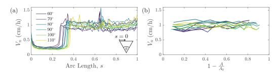
FIG. 8. Dissolution velocity on the lower side is constant with space and time. (a) Dissolution velocity as a function of arc length around a triangular wedge, averaged over time. (b) Average dissolution velocity on the lower side of a triangular wedge as a function of the change in area, normalized by the initial area.
