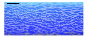
FIG. 6. Small-scale roughness on the underside of a partially dissolved wedge. The wedge has dissolved for 10 min and the scale bar is 1 cm.
