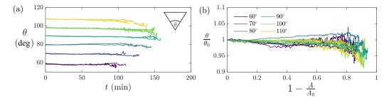
FIG. 7. Shape memory in dissolving wedges. (a) Evolution of the base angle for wedges of differing initial angles. (b) Angle of the wedge normalized by the initial angle as a function of the change in area, normalized by the initial area.
