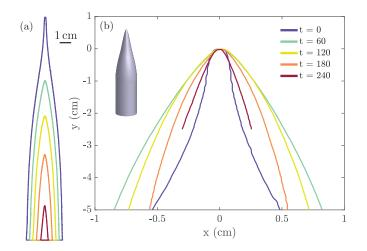
FIG. 14. Sharpened initial shape. (a) Shape profiles shown at 60-min intervals. (b) Zoomed-in, rescaled, and shifted profile shapes to focus on the evolution of the tip. The inset shows a sketch of the initial geometry.
