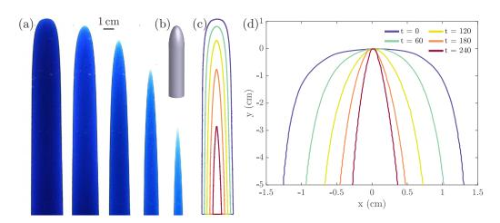
FIG. 13. Shape evolution of a tall axisymmetric body dissolving within water. (a) Photographs shown at 60-min intervals. (b) Sketch of the initial geometry. (c) Extracted cross sections shown every 60 min and at the same scale as images in (a). (d) Zoomed-in and rescaled profiles of the tip region, with all contours shifted to place the tip at the origin.
