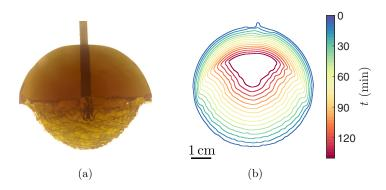
FIG. 1. Shape evolution of a dissolving body. (a) Side-view photograph of candy body (initially a sphere) after dissolution in water for 70 min. (b) Measured profile shape displayed every 10 min. The upper surface remains smooth while the undersurface becomes pitted and dissolves several times faster.
