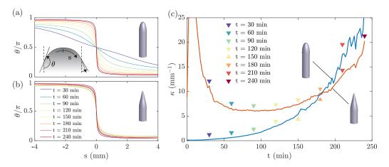
FIG. 15. Tip curvature continuously increases at later times. The angle  $\theta$  of the surface with respect to gravity is plotted vs arc length *s* near the tip for (a) an initially blunt body and (b) a sharpened body. (c) Time evolution of the principal curvature  $\kappa(s = 0)$  at the tip for initially blunt (blue) and sharpened (orange) bodies.
