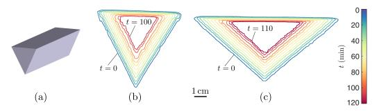
FIG. 5. Shape preservation of dissolving wedges. (a) Sketch of initial configuration: cross-sectional shape evolution at 10-min intervals for bodies with initial base angle (b)  $\theta_0 = 60^\circ$  and (c)  $\theta_0 = 100^\circ$ .
