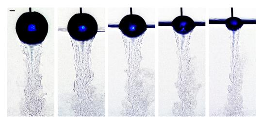
FIG. 2. Shadowgraph images of a dissolution within water at t = 0, 30, 60, 90, and 120 min. The intensity variations beneath the body correspond to a turbulent descending jet of solute-laden fluid. The dark horizontal stripe near the midheight of the body corresponds to the interface of a sharp density stratification. The scale bar is 1 cm.
