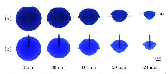
FIG. 3. Tank size has little affect on shape dynamics. Images of dissolving body for (a) tank volume  $180 \text{ cm}^3$  and (b) tank volume  $150 \times 10^3 \text{ cm}^3$ . The stratification interface formed in the smaller tank of (a) causes an optical distortion (dashed lines and arrow) and in reality the bodies are not noticeably different.
