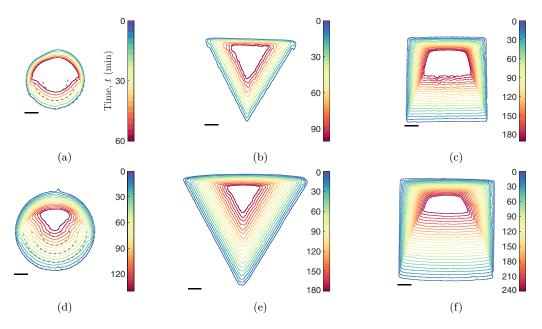
FIG. 11. Comparing shape evolution of quasi-2D and 3D bodies. The initial shapes correspond to those of Fig. 10, with (a)–(c) 2D cylindrical geometries and (d)–(f) 3D solids of revolution. The wedge and cone have  $60^{\circ}$  base angle. In all cases, cross-sectional profiles are shown every 10 min and the scale is 1 cm.
