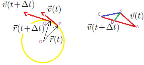
To find the difference of two velocities, we shift  $\vec{v}(t)$  and  $\vec{v}(t + \Delta t)$  so that the two tails are coincide, so the blue line  $\vec{BC} = \vec{v}(t + \Delta t) - \vec{v}(t) \approx \vec{a}\Delta t$ . Now mark a point  $D$  on  $\vec{AC}$  such that  $\vec{AD} = \vec{AB} = |\vec{v}(t)|$ . Now we find that  $\Delta POQ \sim \Delta BAD$ , because both are isosceles and  $\angle POQ = \angle BAD$ . That is because  $\vec{OP} \perp \vec{AB}$  and  $\vec{OQ} \perp \vec{AD}$ .
