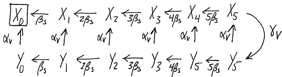
The system moves to the absorbing state  $X_5$  and stays there. Thus the channel is closed with all subunits in state S and the membrane release site is occupied by a vesicle.
