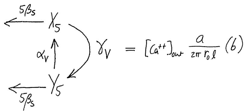
in which the system is known to be in the state  $X_5$  at  $t=0$ . We are interested in the number of vesicle release events which occur before the system exits to the left. (Each release event is a transition along the arrow labeled  $\gamma_V$ .) To find the probability distribution of this number, we relabel the foregoing diagram in terms of probabilities
