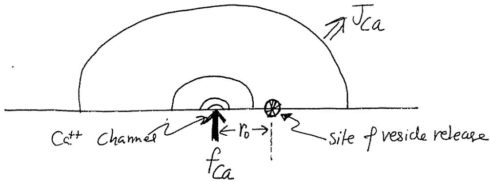
Let the flux through the channel be  $f_{Ca}$ . For an open channel, we previously found
