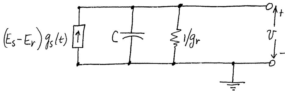
Thus, for small synaptic conductance, the deviation from rest of the membrane potential behaves like the response of a parallel RC circuit to a current source equal to  $(E_s - E_r)g_s(t)$ . This is excitatory if  $E_s > E_r$  and inhibitory if  $E_s < E_r$ .
