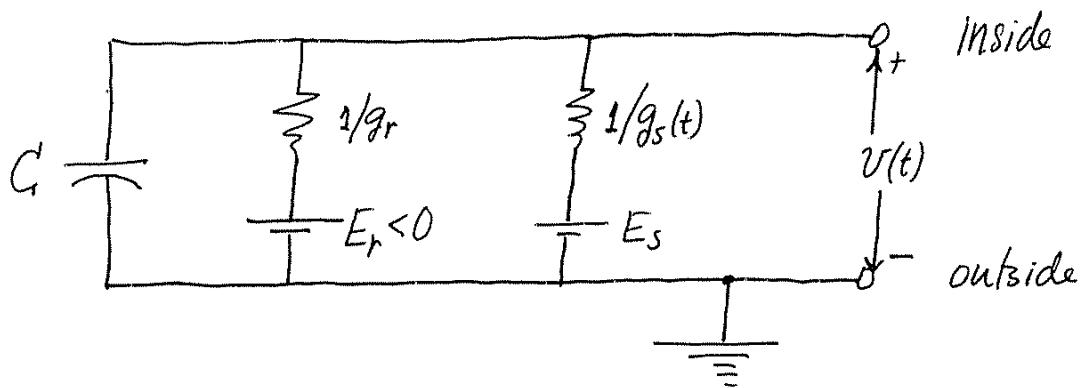
The postsynaptic membrane can be modeled by the foregoing circuit, in which
