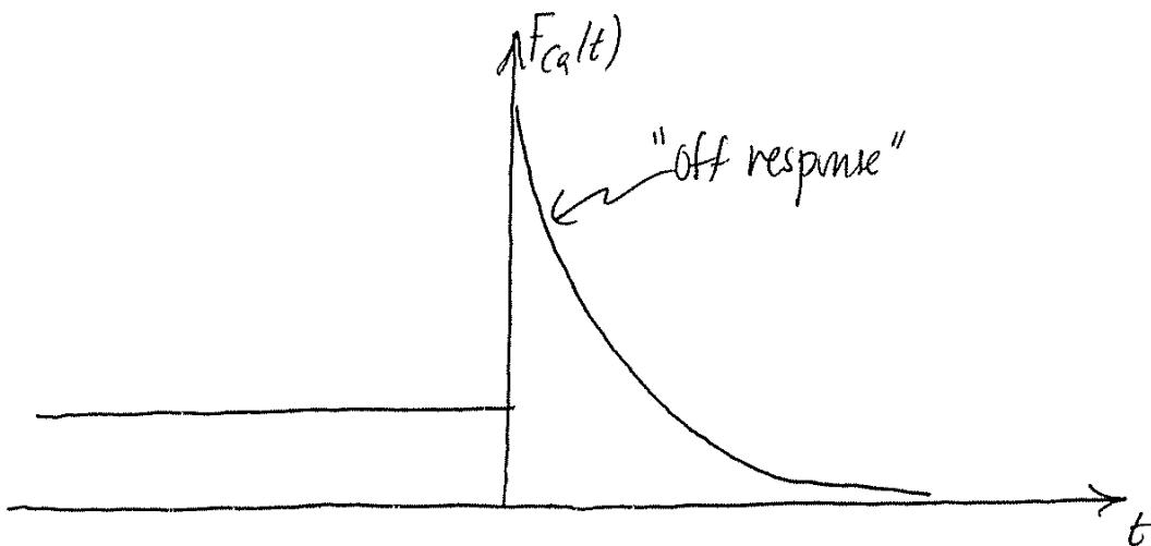
Thus, there is a large burst of  $Ca^{++}$  current following a downward step in voltage that ultimately turns the  $Ca^{++}$  current off.
