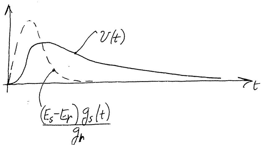
Because of the membrane capacitance, the postsynaptic voltage has a longer tail than the synaptic conductance change.
