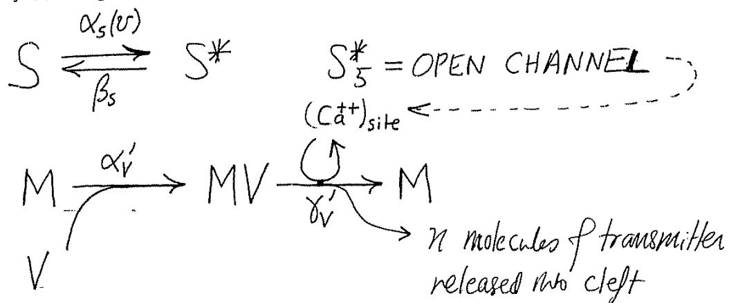
Here  $S$  denotes one of the 5 subunits of the  $\text{Ca}^{++}$  channel; when all 5 subunits are in the state  $S^*$ , the channel is open and  $\text{Ca}^{++}$  appears at the vesicle release site, which is denoted by  $M$ . The free vesicles are denoted  $V$ , and  $MV$  represents a site with a vesicle bound, ready for release. When release occurs, the vesicle is destroyed, the
