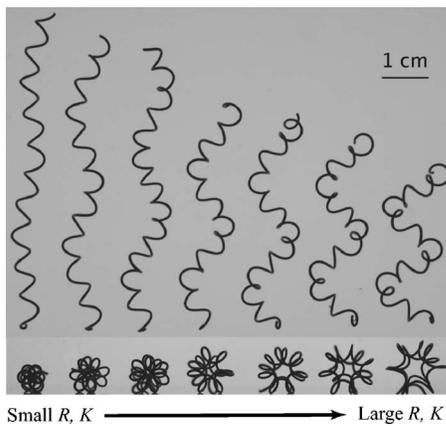
FIG. 3. Seven superhelices with increasing axial helix radius (from left to right). The upper panel is the side view and the lower panel is the axial view. Radius ( $R$ ) and wavenumber ( $K$ ) of the axial helix. As the initial coil is pulled apart, the radius and wavenumber of the axial helix increase. This relation can be predicted by the simple scaling relation with inextensibility of a wire.
