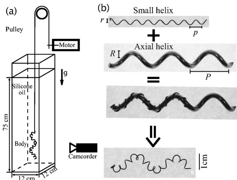
FIG. 2. (a) Schematic of experimental setup. A motor pulls a rigid body through silicone oil, a highly viscous Stokes fluid ( $\nu=10\,000$  cSt). (b) Procedure for making superhelix.
