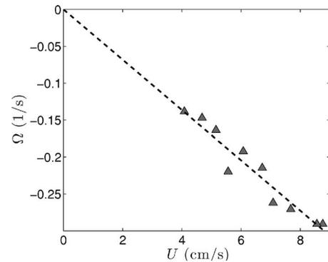
FIG. 4. A linear relationship between the translational velocity and rotational frequency of a superhelix ( $r = 0.89$  mm,  $R = 4.62$  mm,  $p = 5.5$  mm, and  $P = 19.4$  mm). Triangles are from experimental observations. Dashed line is a least-squares fit of experimental data.
