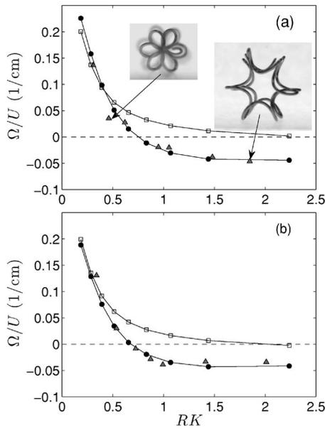
FIG. 5. Ratio of angular velocity to translational towing velocity. Triangles are values measured experimentally. Circles connected by lines are values predicted using the method of Regularized Stokeslets. Squares are values predicted using resistive force theory. (a) Superhelices of set I. Positive rotational rate is clockwise and negative rate is counterclockwise. Rotational direction changes around 0.7 for  $RK$ . (b) Superhelices for set II. Same transition also occurs around 0.7 for  $RK$ .
