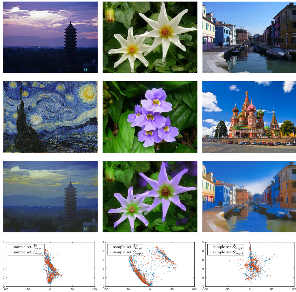
FIGURE 4.8. More color transfer examples, with source images on the top row, targets on the second row, and the results of transferring on the third. The bottom row displays the sample points of the target and those of the transformed source.
