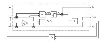
Fig. 4. Block diagram of the Golden Ratio Encoder (Section III) corresponding to the DAG model in Fig. 2.
