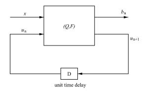
Fig. 1. Block diagram describing an algorithmic encoder.
