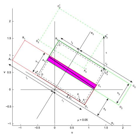
Fig. 6. Positively invariant set and the demonstration of its robustness with respect to additive noise and imperfect quantization.
