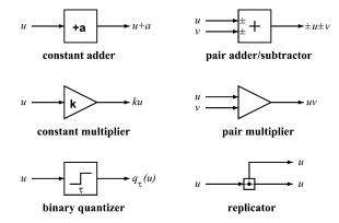
Fig. 3. Representative class of components in an algorithmic encoder.
