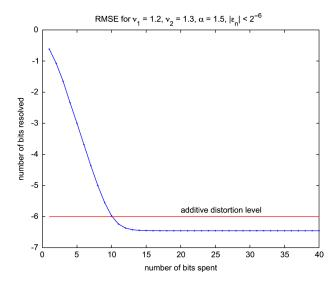
Fig. 8. Demonstration of the fact that reconstruction error saturates at the noise level. Here the parameters are  $\nu_1 = 1.2$ ,  $\nu_2 = 1.3$ ,  $\alpha = 1.5$ , and  $|\epsilon_n| < 2^{-6}$ .
