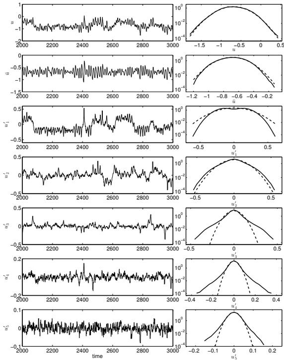
**Fig. 2.** Positive large scale damping : time series (left column) and pdfs (right column) of the turbulent signal  $u, \bar{u}$  and  $u'_k, k = 1, 2, \dots, 5$  with  $\bar{F} = -0.080$ . Note the logarithmic scale of pdfs in the y-axis. Dashed lines are Gaussian distributions with the same mean and variance.
