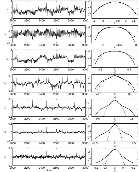
**Fig. 1.** Negative large scale damping : time series (left column) and pdfs (right column) of the turbulent signal  $u$ ,  $\bar{u}$  and  $u'_k$ ,  $k = 1, 2, \dots, 5$  with  $\bar{F} = -0.055$ . Note the logarithmic scale of pdfs in the y-axis. Dashed lines are Gaussian distributions with the same mean and variance.
