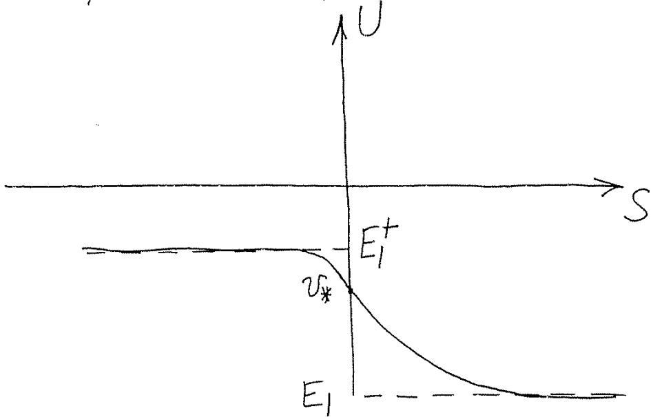
$$U(S) = \begin{cases} E_1^+ + (v_* - E_1^+) \exp(\lambda S) & S < 0 \\ E_1 + (v_* - E_1) \exp(\mu S) & S > 0 \end{cases}$$
