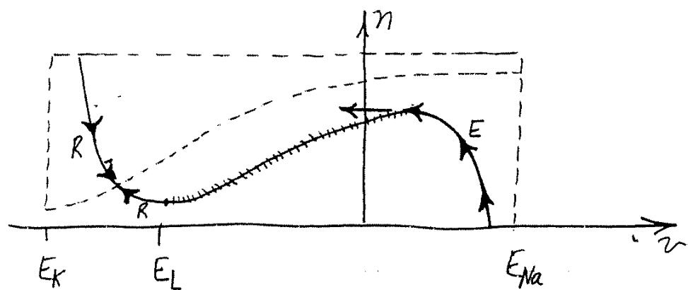
An action potential can now be understood as follows. The rest state of the neuron is the intersection of the curve  $f(n, v) = 0$  (the slow manifold) with the curve  $n = n_{\text{ss}}(v)$ . Let a neuron be at rest there and let a current pulse be applied which is sufficient to step the voltage across the T branch of the slow manifold. Then the neuron jumps to the E manifold, where it evolves to the top, jumps back to the R manifold, and then recovers to its starting point.
