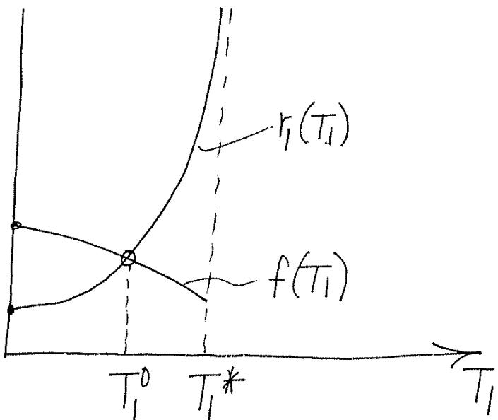
Thus  $T_1 = T_1^0$  is the duration of the pulse. Note that  $T_1^0 < T_1^*$ , the time at which the excited state would reach threshold. The pulse "jumps" across threshold on the downstroke just as on the upstroke. (It looks more and more like a jump as  $\epsilon \rightarrow 0$ .)
