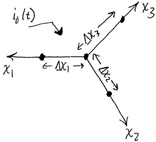
Since the voltage is continuous at a junction, we only need one node there. Let the junction voltage be denoted  $V_0(t)$ . This takes care of Eq. 26.
