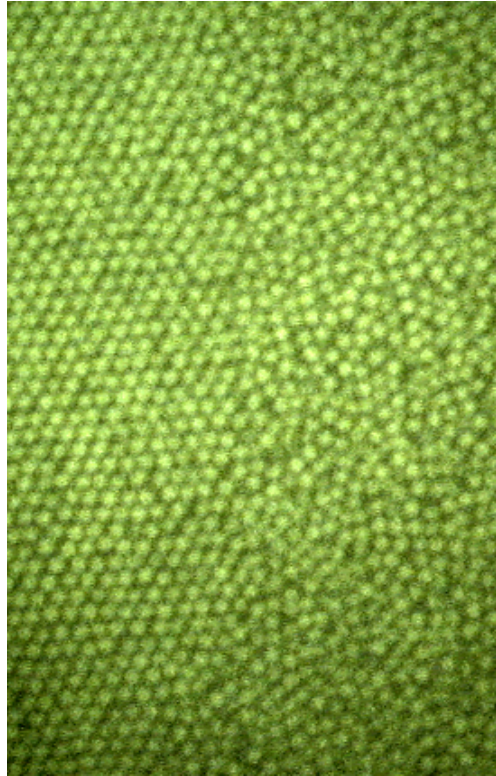
Figure 1.2: ( Left ) A carefully arranged ordered packing of ball bearings surrounded by a disordered pile of bearings, taken from Ref. [42]. ( Right ) [Courtesy of Paul Chaikin] A colloidal system of spherical particles in an external electric field, causing a density gradient from a less dense disordered liquid structure (right), to a more dense ordered crystal structure (left).
