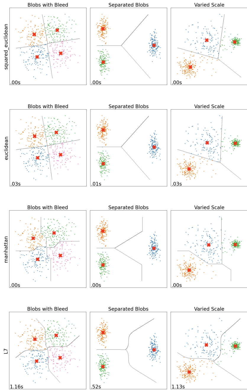
Figure 3: Demonstrating the k -GenCenters module on three toy datasets. Using squared_euclidean and euclidean costs, the first two rows show k -means and k -medians, respectively. A red x shows the final position of each center, coloration of the data shows the final assignments, Voronoi boundaries are drawn in black, and runtime is printed in the southwest corner of each plot.
