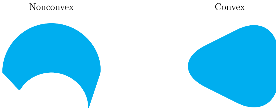
Figure 9: An example of a nonconvex set (left) and a convex set (right).
