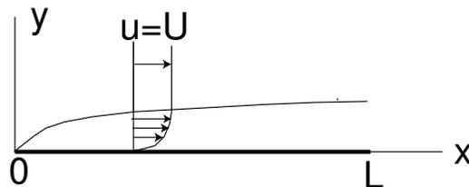
Figure 8.1: Boundary layer on a finite flat plate.
