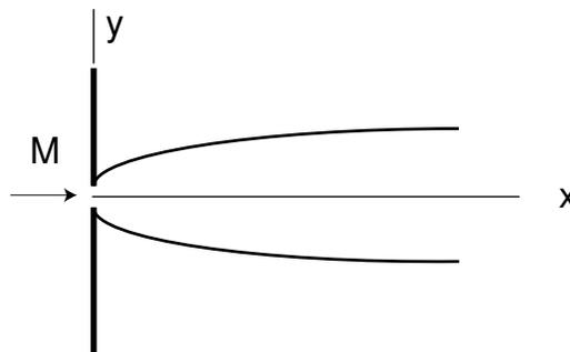
Figure 8.5: A two-dimensional laminar jet emerges from a slit in a wall.
