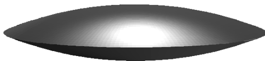
FIGURE 6.1. Three-dimensional sketch for the (expected) total shape for inclusions with large volume.
