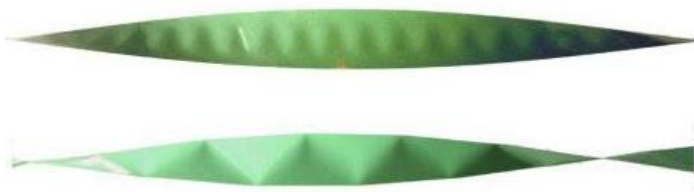
Fig. 2: Twisted mylar ribbons: experimental results from [11]. Used with permission.
