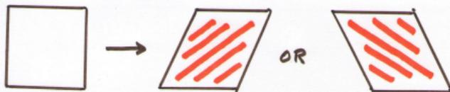
Substrate prohibits large deformation; therefore the film mixes the two shear-combined-with-wrinkling variants. Thus, the **herringbone pattern has two length scales:**
