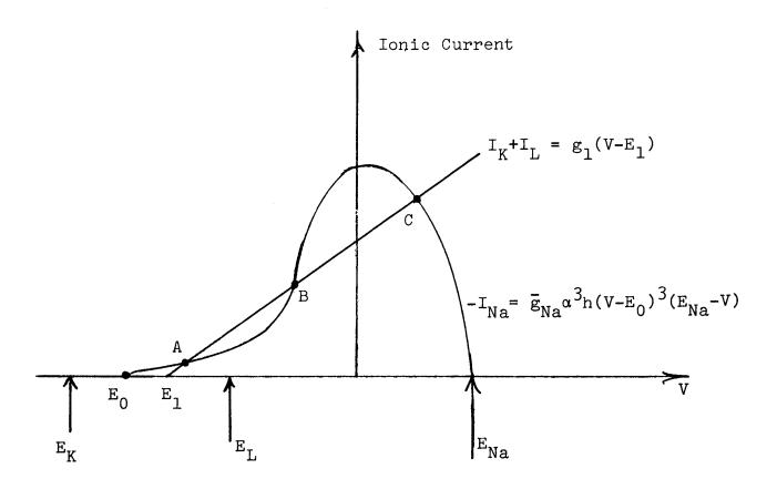
The points A, B, C are the points where dV/dt = 0. Reference to the sign of dV/dt in the neighborhood of these points shows that A and C are stable, while B is unstable. If V > B,  $V \to C$ , but if V < B,  $V \to A$ . Therefore B is a "threshold", spearating two stable states which may be called the <u>resting state</u>, A, and the excited state C.
