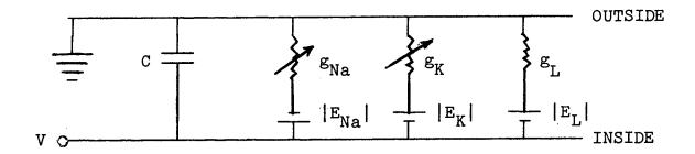
The "batteries"  $E_{Na}$ ,  $E_{K}$ ,  $E_{L}$  have e.m.f.'s which are determined by the appropriate ratios of ionic concentrations. For example
