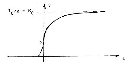
This solution is a "change of state" wavefront, traveling to the left with velocity  $\theta$ . Each section of the line is brought to threshold a by diffusion, whereupon it turns on and drives itself to the excited state  $E_0$ .
